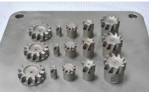
Multiple AM cutter parts produced on a single build plate.
