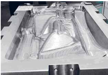
3D pre-Milled Dash board Mold
